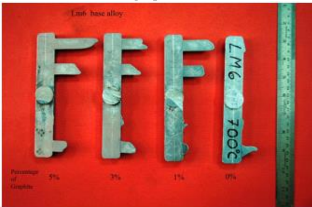
Fig.14 Variation of strip fluidity length with % graphite
