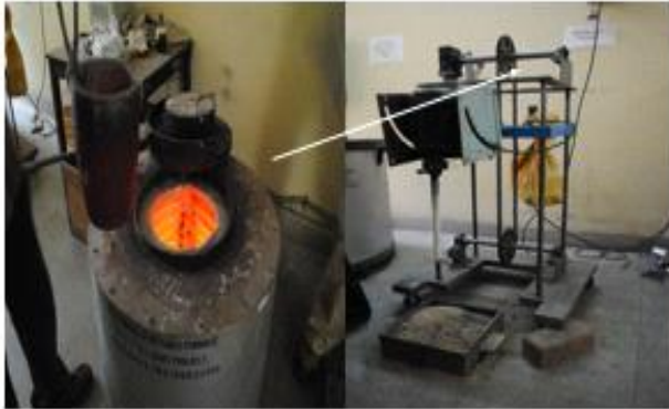
Fig.1 9kW electric resistance furnace and stirrer setup
