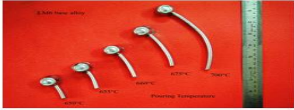
Fig.6 Variation of Aluminium LM6 spiral fluidity length with temperature
